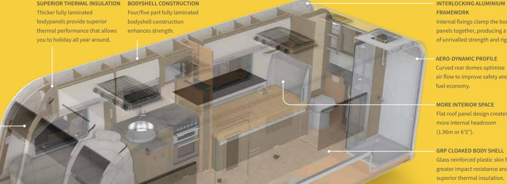
Internal fixings clamp the body panels together, producing a shell of unrivalled strength and rigidity.
