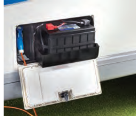
105Ah auxiliary battery
