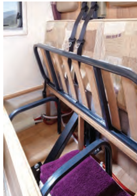
Additional strengthening to furniture in dedicated rear passenger area (745 & 760 only)
