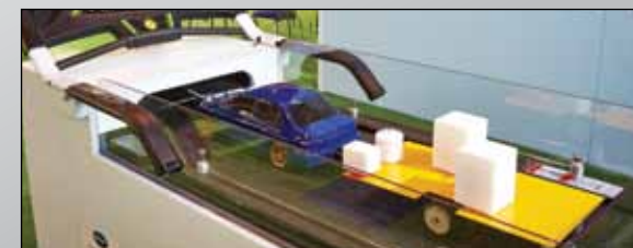
Above: The towing stability model developed by University of Bath shows how a trailer's stability varies according to the location of heavier items such as the gas bottle and battery.
