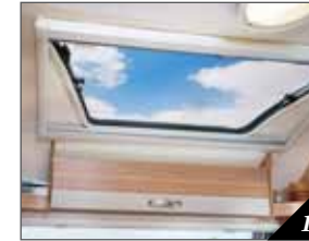
1) Polyplastic double glazed opening sunroof with night blind in front dome. 2) AL-KO ATC Trailer Control System.
